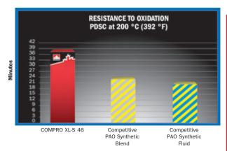
COMPRO XL-S provides excellent resistance to oxidative breakdown caused by exposure to air at high temperatures.
