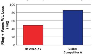
†Test duration: 100 h/cartridge; Outlet pressure: 3200 psig; Inlet temperature: 104 °C (220 °F) Four ASTM D943 copper & iron coils added to reservoir for 200 h
