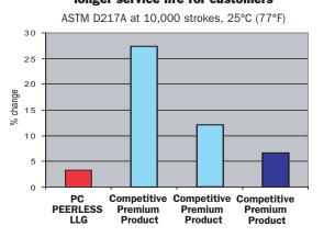
\* The significance of the tests is to demonstrate the stability of the grease under normal and moderate shear conditions. The lower the number in the graph, the stronger the grease performance, and the longer its service life.
