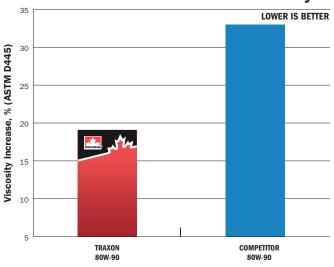
In the L-60-1 oxidation test, product performance is measured by how much harmful viscosity increase will occur over time (therefore, the lower the bar the better). Compared to this competitor, TRAXON 80W-90 with its advanced formulation is clearly superior.
