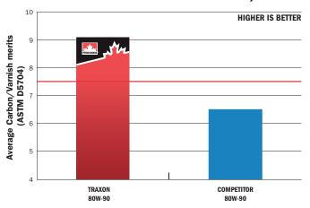
In the standard L-60-1 oxidation test, product performance can be measured by how clean the gear parts are after being exposed to a lubricant and high temperature. A merit system has been standardized from 1 to 10 (10 being pristine and 7.5 or lower being unacceptable for an SAE J2360 qualified fluid). Compared to this competitor, TRAXON 80W-90 has outstanding gear surface cleanliness and far exceeds the minimum SAE J2360 standards.
