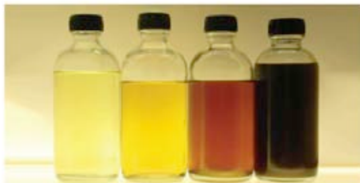
FIGURE 4: Progressive discoloration occurs when a heat transfer fluid is exposed to oxygen over time.
