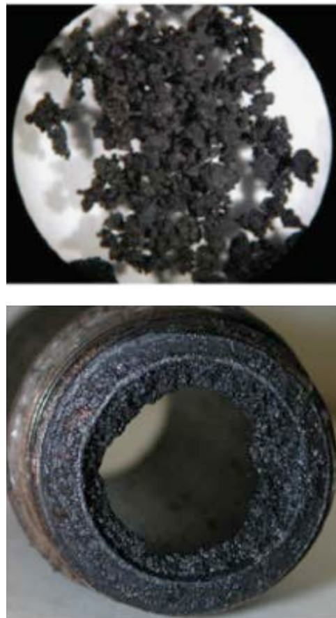
FIGURE 2a/b: A hydrocarbon in a mineral-based heat transfer fluid undergoes thermal degradation, which creates lighter hydrocarbons with lower viscosities and flash points, and heavy carbon deposits (FIGURE 2b).
