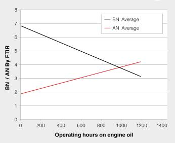
BN and AN cross over is a typical indication of the need to change the oil. DURON HP 15W-40 demonstrates up to 1,000 hr drain extensions
