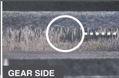
Heavy scuffing on all pinion teeth. Failed load stage 9 due to excessive wear. Minimal cross hatching remaining.
