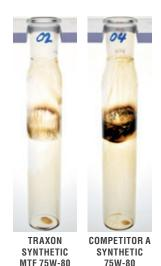
TRAXON Synthetic MTF 75W-80 shows excellent oxidation and thermal stability versus Competitor A as shown above. Indication of better surface cleanliness with reduced sludge and deposit demonstrates how it can help transmissions run at optimum efficiency.
